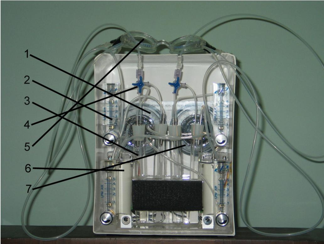
Figure 1: One of the two identical airflow systems that constituted the exposure device
