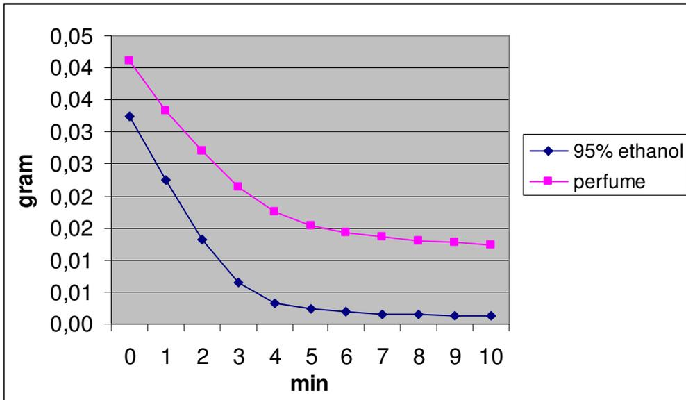
The time dependent fall in weight when evaporating 50  $\mu$ L perfume and 50  $\mu$ L 95% ethanol for 10 minutes. The units of measurement are average delta values based on 10 measurements.
